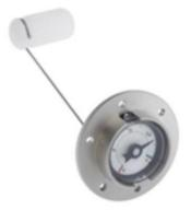
The **G/LL 28 Series** is a simple, robust, mechanical liquid level contents gauge using a float to move the dial pointer via a magnetic coupling. This prevents ingress of the tank contents into the indicator capsule.
