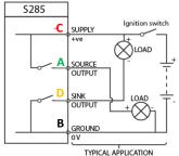
NOTE: IF SINK ONLY OUTPUT IS REQUIRED THEN PIN A IS NOT USED.
